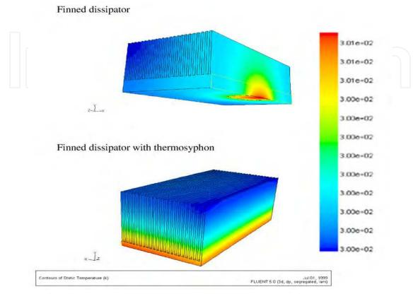
Fig. 5. Temperature distribution in a finned dissipator, with and without thermosyphon.
