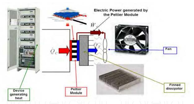
Fig. 12. Sketch of a thermoelectric self-cooling system.
