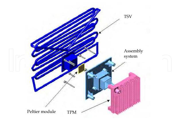
Fig. 10. Thermoelectric device with the heat exchangers TSV and TMP.
