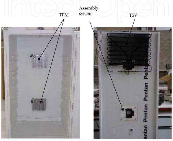
Fig. 11. Photographs of the prototype with heat exchangers TMP and TSV.
