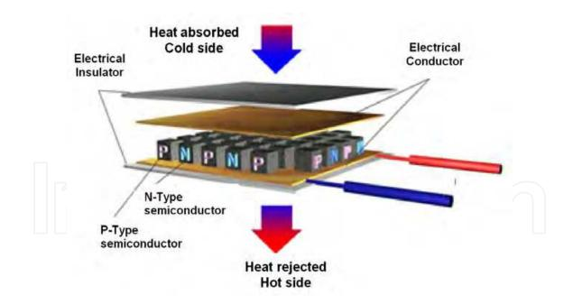
Fig. 1. Sketch of a Peltier module working as refrigerator.
