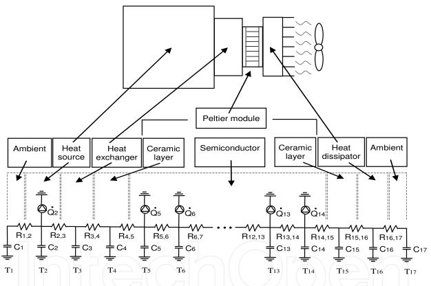
Fig. 3. Sketch and discretization of a thermoelectric generator.
