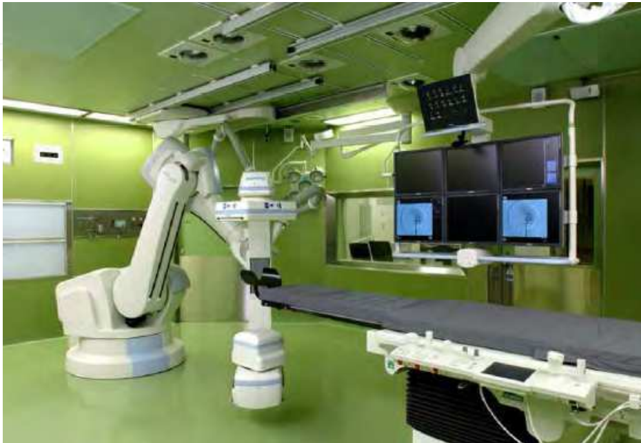
Fig. 11. Siemens robotic surgical C-Arm system Artis zeego
