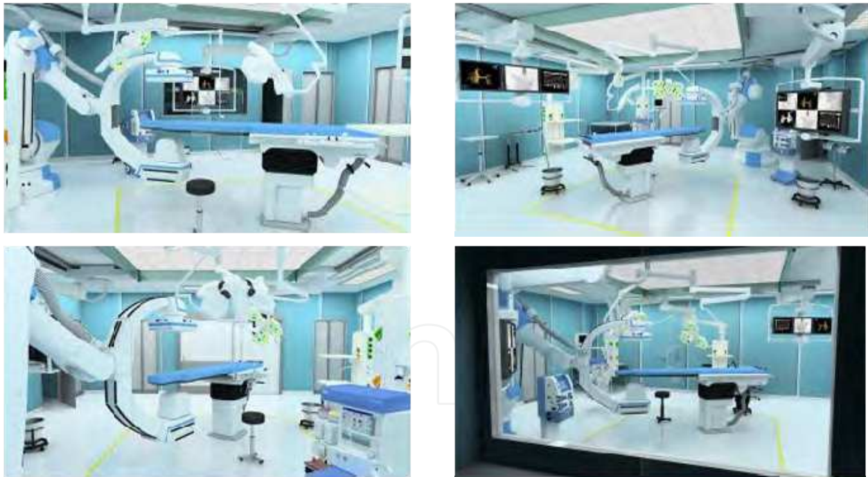
Fig. 19. Examples for 3D presentation of a hybrid OR plan, ensuring a common vision of the future facility across all parties involved
