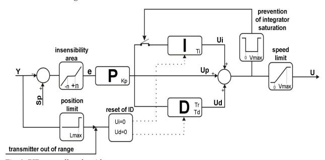
Fig. 3. PID controller algorithm
