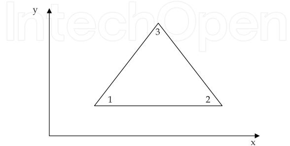
Fig. 4. Linear triangular finite element
