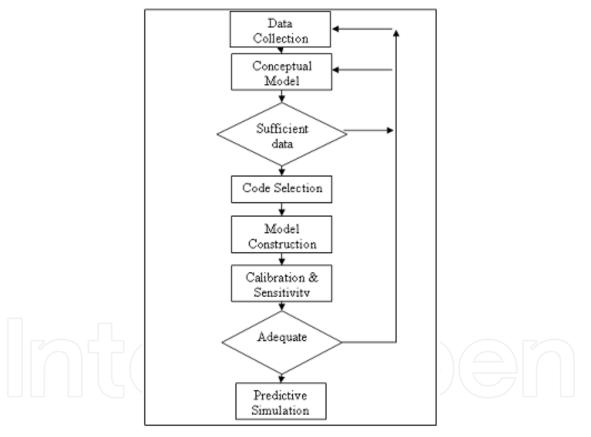
Fig. 3. Groundwater flow methodology (ASTM, D5447-2004)
