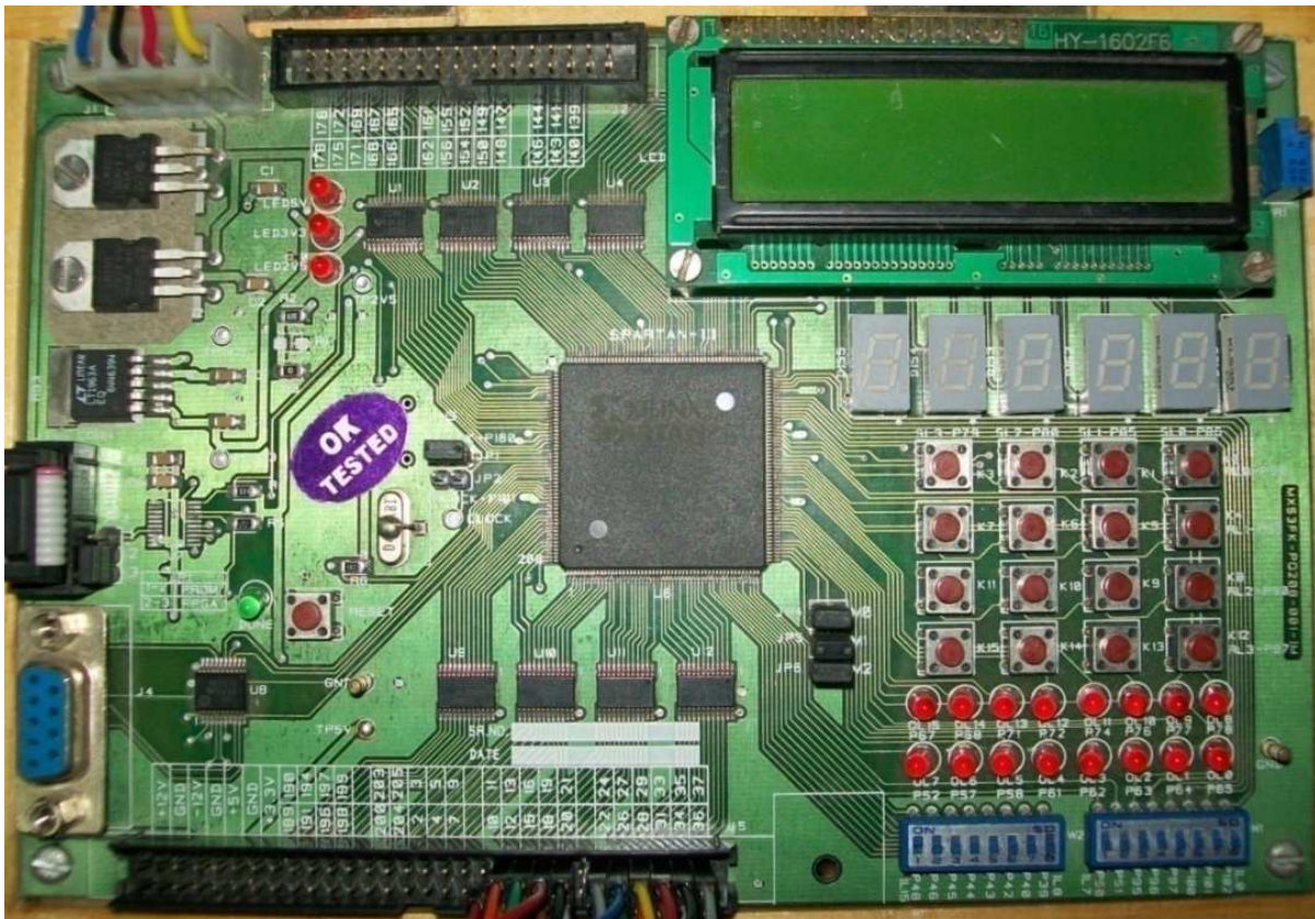
Fig. 8. XILINX SPARTAN3 FPGA Kit
