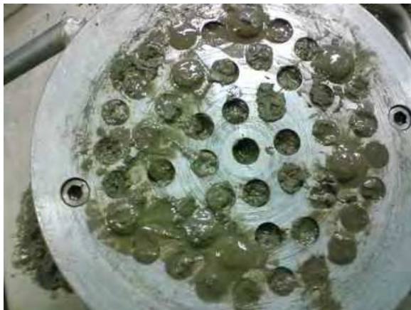
(a) The water within cement-based composite was drained out
