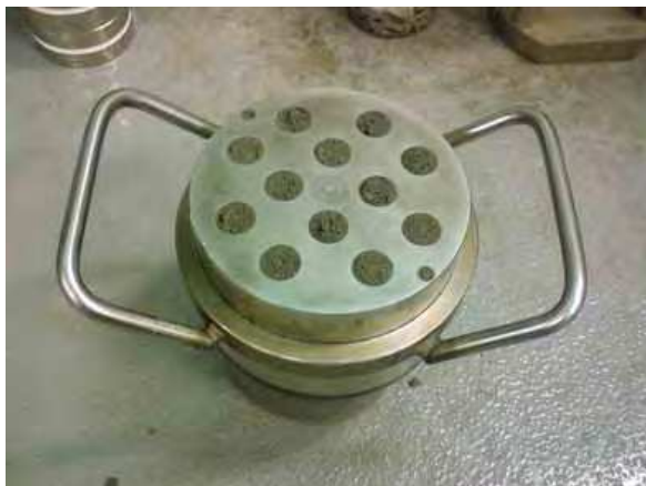
(a) Step 1: To fill the mixed cement-based composite into the mold
