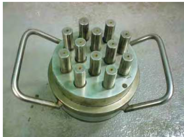
(b) Step 2: To set up the pestle into the mold into the mold
