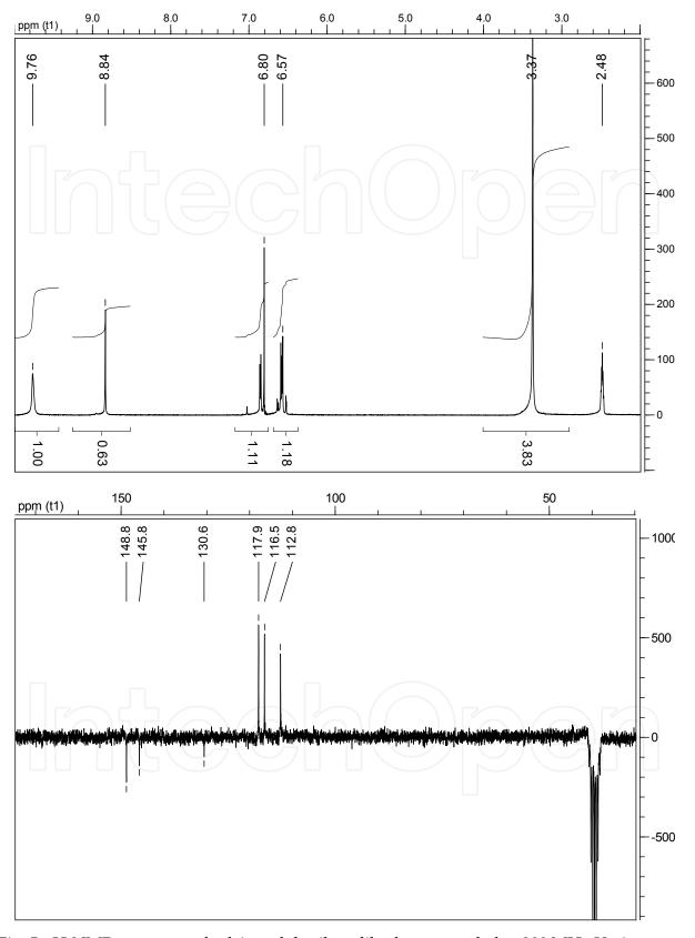
Fig. 5.  $^{1}$ H-NMR spectrum of calcium dobesilate dihydrate recorded at 200 MHz Varian Gemini FT-NMR spectrometer in DMSO-D<sub>6</sub> solution (top) and its  $^{13}$ C-NMR spectrum measured in DMSO-D<sub>6</sub> solution at 50 MHz at the same instrument (bottom).
