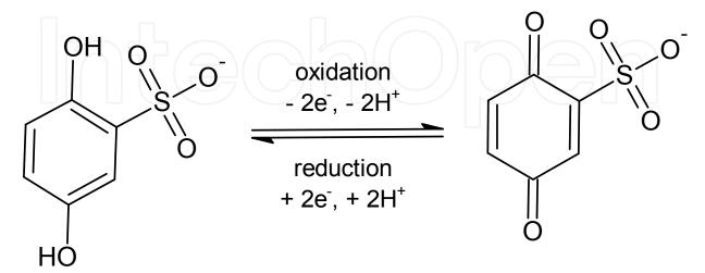
Fig. 7. Reversible oxidation of dobesilate anion into 3,6-dioxocyclohexa-1,4-diene-1-sulfonate.
