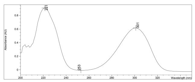
Fig. 6. Ultraviolet spectrum of calcium dobesilate measured in an aqueous solution at Agilent 8453 diode array UV-VIS spectrophotometer in accordance with requirements of the European Pharmacopoeia (European Pharmacopoeia Edition 7.2, 2011).
