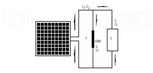
Fig. 14. The diagram of data acquisition circuit
