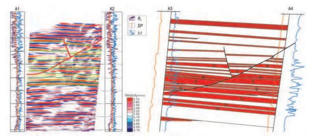
Fig. 4. Application of inter-well seismic survey for reservoir prediction in some oilfield, China. The picture on the left shows the result of ineterwell seismic imaging and the right one is about interwell seismic interpretation. It illustrates that interwell reservoir heterogeneity can be investigated and small scale faults can be identified clearly.
