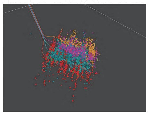
Fig. 2. Perspective view of the microseismic monitoring results from treating five wells completed in the Marcellus Shale in Pennsylvania. The dots represent the estimated event hypocenters. The colors of the dots match the color of the treated well to which they correspond. (From Schisselé and Meunier, 2009; Duncan and Eisner, 2010).
