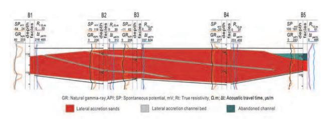
Fig. 5. Cross-section profile for reservoir architecture of single channel sand in a block of Daqing Oilfield, China. Sand lateral accretion can be identified and subdivision of the single point bar into multiple lateral accretionary sands was initialized. It further reveals that genetic units inside reservoir architecture are separated or laminated.
