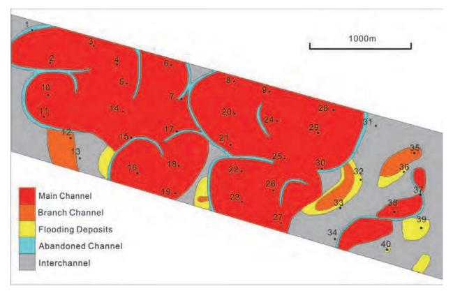
Fig. 3. Microfacies distribution of P I31 sub-layer in a block of Daqing oilfield, China
