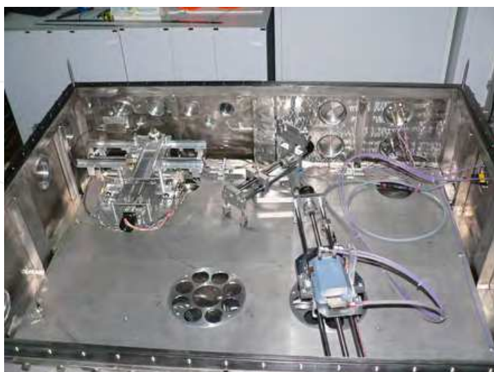
Fig. 2. Inside view of the J. Stefan Institute's WDX spectrometer vacuum chamber with the target holder on a goniometer, crystal holder, and the CCD camera. A mechanical theta/2theta stage serves to adjust the Bragg angle.
