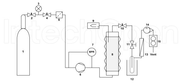
Fig. 1. Schematic diagram of a lab scale SC-CO<sub>2</sub> extraction system: 1, CO<sub>2</sub> tank; 2,4,10, shut-off valves; 3, pressure gauge; 5, filter; 6, compressor; 7, back pressure regulator; 8, extraction vessel; 9, thermocouple; 11, micrometering valve; 12; sample collector; 13, oil and moisture trap; 14, flowmeter; 15, gas meter.
