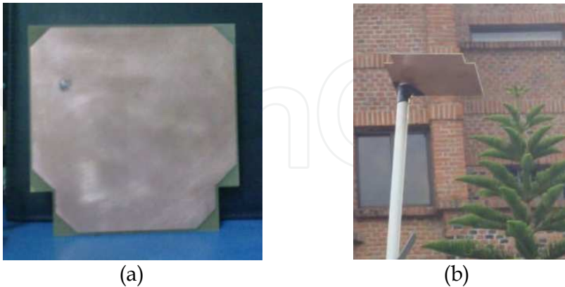
Fig. 10. (a) Patch antenna array prototype. (b) Prototype mounted on a PVC base, outdoors of the CIICAp building.
