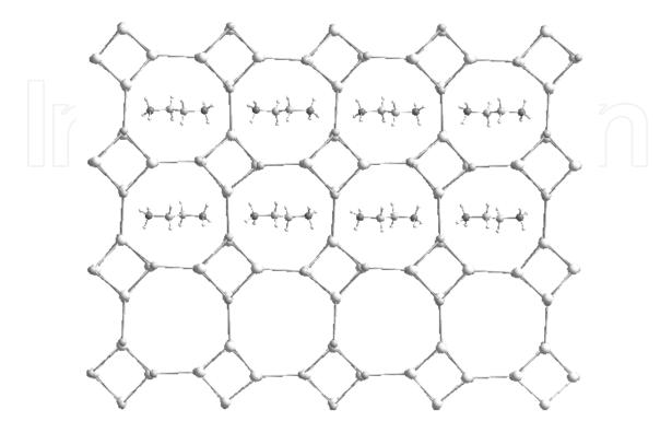
Fig. 8. CoZnPO<sub>4</sub>-II seen along [001] direction showing the stacked 4.8<sup>2</sup> nets to form 3D framework and 8-ring with diprotonated ethylenediame cations accommodated in the channel (each node is a T-atom, oxygen atoms are omitted for clarity).
