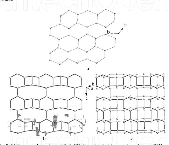
Fig. 7. (a) The crystal structure of  $CoZnPO_4$ -I consisted of 6-rings viewed down [001]; (b) A sheet extends along the (010) plane consisted of 4-, 6-, and 10-rings;(c) The sheets stacked along the direction vertical to the (010) plane (each node is a T-atom, oxygen atoms are omitted for clarity).
