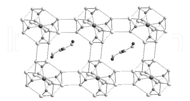
Fig. 9. CoZnPO<sub>4</sub>-III I seen along [100] direction showing the 8-ring channels with diethylenetriaminum cations accommodated in the channel.
