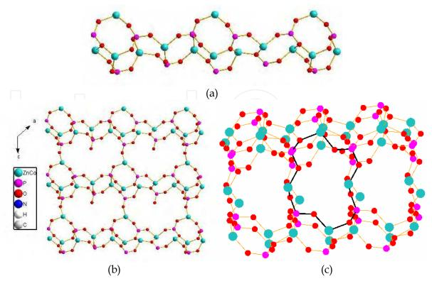
Fig. 2. (a) The secondary structural unit of CoZnPO<sub>4</sub>-IV; (b) Structure of 10-rings along *ac*-plane in CoZnPO<sub>4</sub>- IV; (c) Structure of 8-ring channel in CoZnPO<sub>4</sub>- IV.
