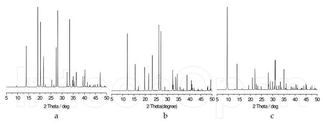
Fig. 6. XRD patterns of three cobalt-zinc phosphates: (a) CoZnPO<sub>4</sub>-I; (b) CoZnPO<sub>4</sub>-II; (c) CoZnPO<sub>4</sub>-III.
