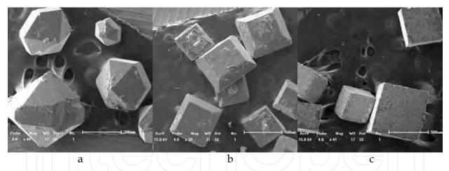
Fig. 5. SEM images of the large crystals of three cobalt-zinc phosphates : (a) crystal of CoZnPO<sub>4</sub>-I with elongated hexagonal-dipyramid morphology;(b) CoZnPO<sub>4</sub>-II crystal with square bifrustum morphology; (c) CoZnPO<sub>4</sub>-III crystal with cubical-like morphology.
