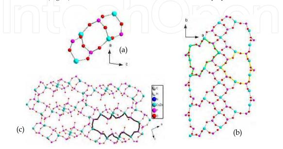
Fig. 3. (a)  $4^3$  unit along b-axis in CoZnPO<sub>4</sub>-V; (b) Structure of 10-rings along *ab*-plane in CoZnPO<sub>4</sub>-V. (c) Structure of 16-rings along *ac*-plane in CoZnPO<sub>4</sub>-V.
