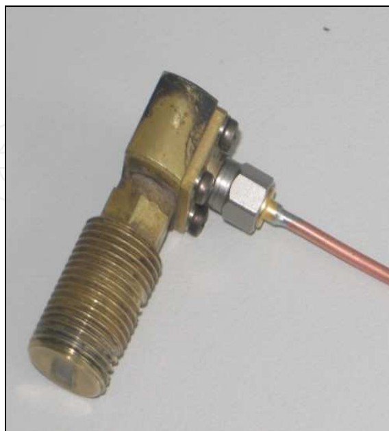
Fig. 20. The antenna for the PIT microwave sensor
