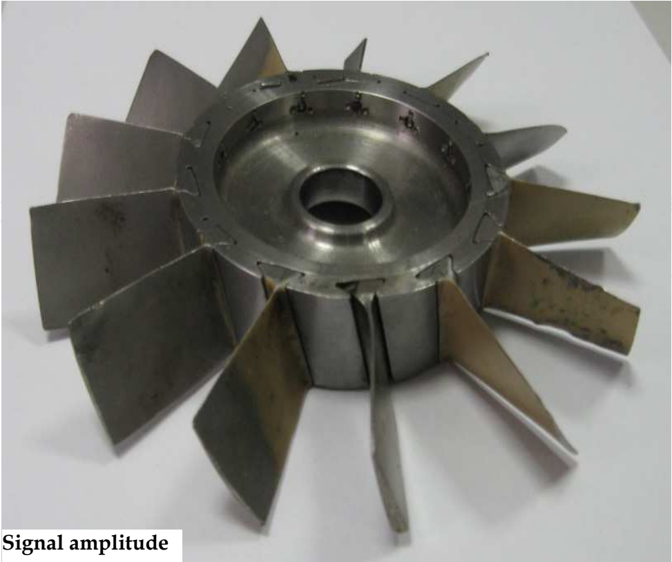
Fig. 8. View of the turbine disc with blades
