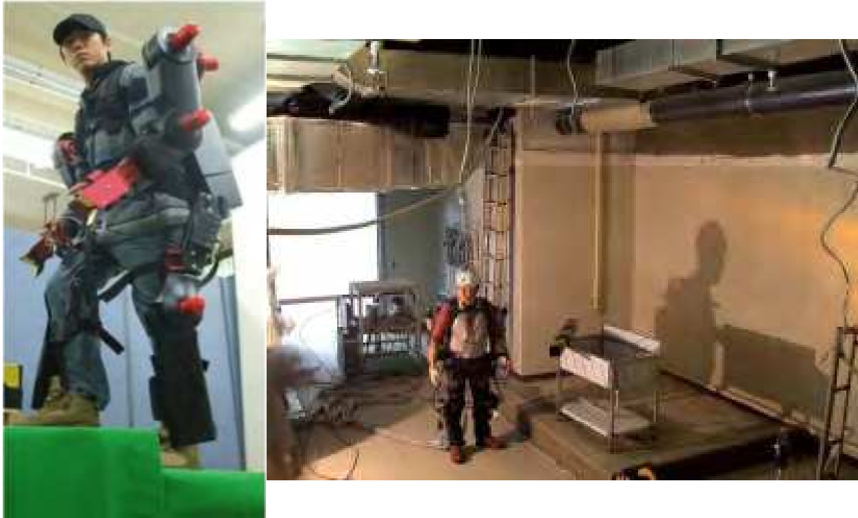
Fig. 10. Wearable robotic exoskeleton system for construction workers. The system can e.g. support workers to carry and assemble heavy steel bars. Hanyang University, Korea
