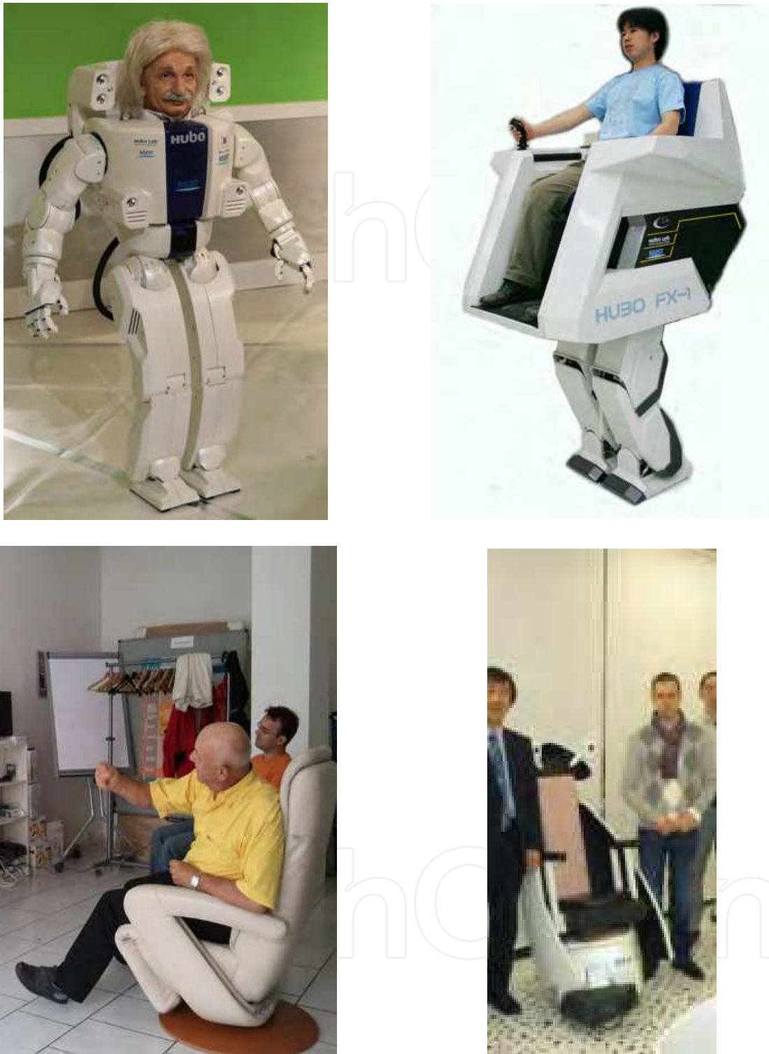
Fig. 19. Similarity and interchangeability of underlying basic technologies between robots of different categories. From left to right: Kaist's Humanoid Robot HUBO, Kaist's Mobile HUBO FX-1 suit built upon the HUBO platform, TUM's GEWOS sensor chair serving as control interface, IRT'S and Toyota's r intuitively controllable robotic wheelchair.
