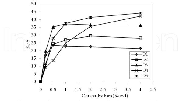
Fig. 5. Build-up curves of azo disperse dyes on PLA fiber (Structures of the dyes are in Table 1.)
