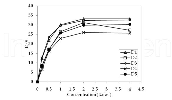
Fig. 6. Build-up curves of azo disperse dyes on PET fiber (Structures of the dyes are in Table 1.)
