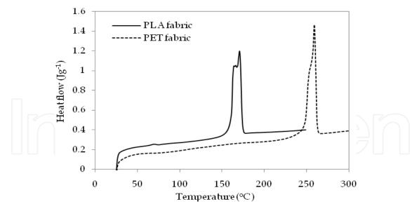
Fig. 2. DSC scans of the knitted fabrics derived from PLA and PET fibers
