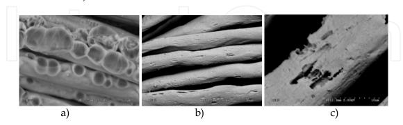
Fig. 3. SEM photographs of damage on PLA fiber caused by ; a) electron irradiation of SEM; b) and c) peroxide bleaching used for PLA/cotton blend
