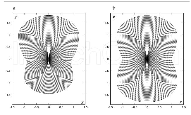
Fig. 8. Reachable sets  $\mathcal{G}^2(t)=G^2(t)$  for system (3),  $t_f=1.8$ ,  $\delta=0.04$ : a) a=-0.8; b) a=-1
