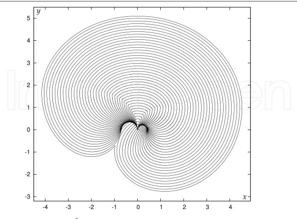
Fig. 12. Reachable sets  $\mathcal{G}_M^2(\tau)=\mathcal{W}(\tau,M)$  for system (4) with a=0.2, b=-0.6. The set M is the circle of radius 0.01 with the center at the origin. The output step of the representation is  $\delta=0.12$ , the terminal time is  $\tau_f=5.21$
