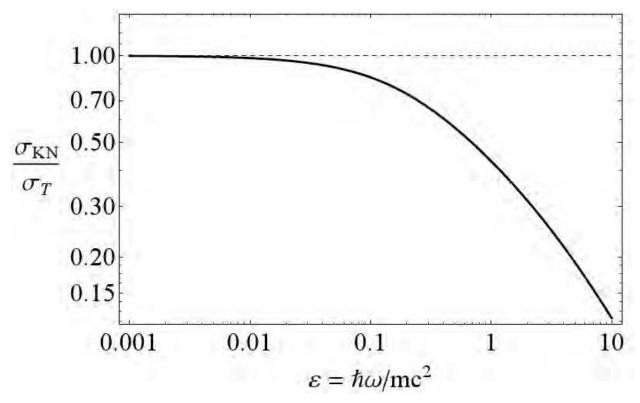
Fig. 1. Plot of the Klein-Nishina expression for the Compton scattering cross section. For small values of  $\varepsilon$ , the Compton cross section approaches the Thomson limit. At large values of  $\varepsilon$ , the Compton cross section approaches the asymptotic solution  $\sigma_{KN} \sim \frac{3}{8} \frac{\sigma_T}{\varepsilon} (\ln 2\varepsilon + \frac{1}{2})$ .
