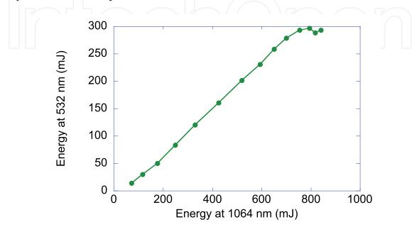
Fig. 21. Frequency doubling of the 10 ps T-REX ILS laser with a peak efficiency of 40%.
