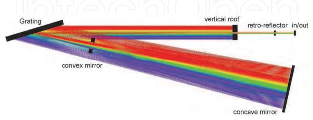
Fig. 9. Raytraced design of the Offner stretcher for the photogun laser.
