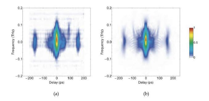
Fig. 17. Experimental measurement of the 800 mJ pulse duration. (a) Field of the experimentally measured FROG spectrogram. (b) Lowest error field obtained by a FROG algorithm using a 512x512 discretization grid.
