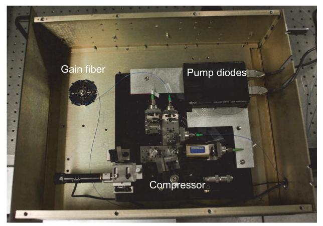
Fig. 10. The ultrashort Yb<sup>+</sup> doped fiber oscillator fits on a  $12'' \times 12''$  breadboard. When recompressed, the anomalous dispersion oscillator generates 100 fs pulses.
