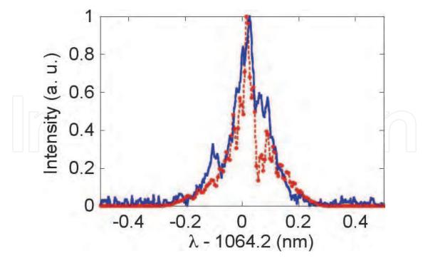
Fig. 19. Pulse spectrum from FROG (red dots) and spectrometer (solid line) measurements.
