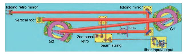
Fig. 16. The compact hyper-dispersion stretcher matches the GDD of the compressor.
