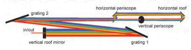
Fig. 14. The compact hyper-dispersion compressor consisting of two 1740 grooves/mm gratings has a footprint of 3x0.7 m and group delay dispersion of -4300 ps<sup>2</sup>/rad.
