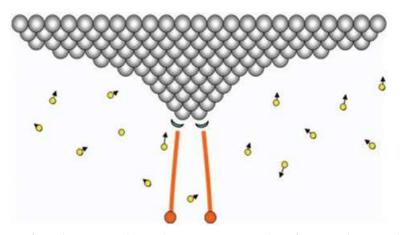
Fig. 4. Spherical tip after the atoms have been rearranged to form a three-sided pyramid. Now the ionization disks exist only over the topmost three atoms. Reprinted with permission from Ward B.W., Notte J.A. & Economou N.P., 2006. Helium ion microscope: A new tool for nanoscale microscopy and metrology. JVST B 24(6), 2871. Copyright 2006, American Vacuum Society.
