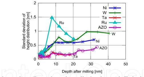
Fig. 16. Impact of ion milling on the roughness of hard mask materials. The hard mask thickness before milling was 10±2 nm in all cases.
