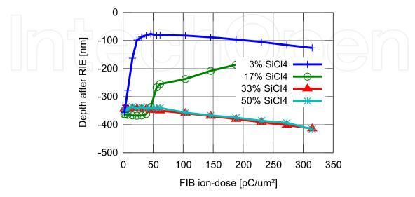
Fig. 17. Impact of the addition of SiCl<sub>4</sub> to the masking capability of Ga implanted by FIB into Si in a SF<sub>6</sub>-based RIE process
