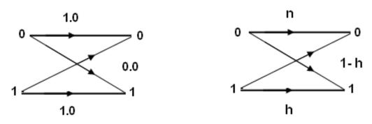
Fig. 4. Transition diagram and bit error probabilities model
