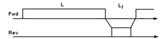
Fig. 3. Block-oriented transmission scheme
