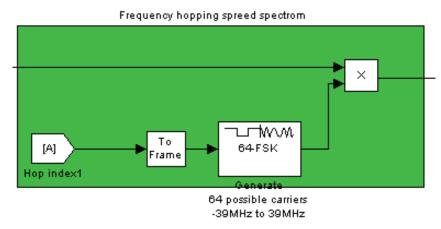
Fig. 8. Design of frequency hopping spreader
