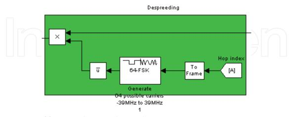
Fig. 9. Design of frequency hopping despreader
