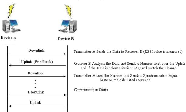
Fig. 1. Shows the communication scheme
