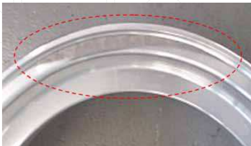
Fig. 8. Wheel distortion after post-cast cooling in water at a temperature of 30°C
