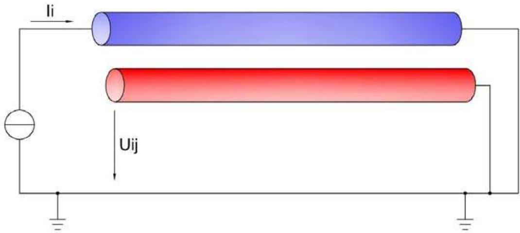
Fig. 5. Mutual impedance calculation
