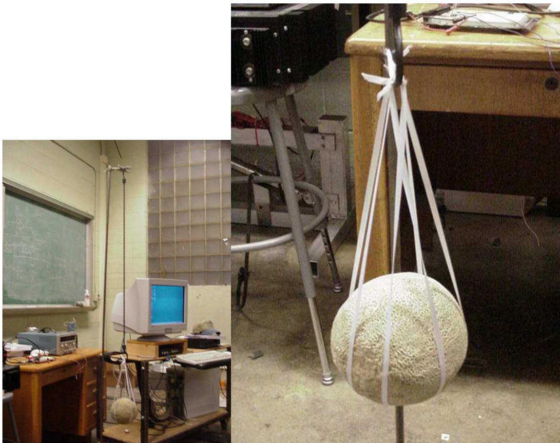
Fig. 19. A long elastic cord and rubber bands supporting the melon.
