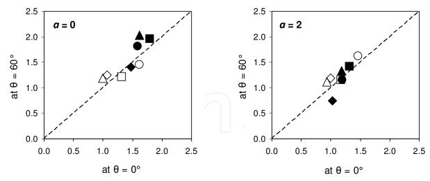
Fig. 8. Plots of  $OH_{inorg}$  /  $O_{529.7}$  ratio measured by XPS at  $\theta = 60^{\circ}$  vs  $\theta = 0^{\circ}$  on native (open symbols) or silanized stainless steel (closed symbols), as such  $(\blacklozenge, \diamondsuit)$  or further treated with coupling agent BS  $(\blacktriangle, \triangle)$ , glucose oxidase  $(\blacklozenge, \bigcirc)$  or coupling agent followed by glucose oxidase  $(\blacksquare, \square)$ . The dashed lines represent a y/x ratio of 1:1.
