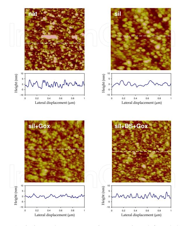
Fig. 1. AFM height images ( $1 \times 1 \mu m^2$ , contact mode, in water; z scale 10 nm) of native (nat), silanized stainless steel (sil), the same after adsorption of glucose oxidase (sil+Gox) and after treatment with glucose oxidase subsequent to treatment with the coupling agent (sil+BS+Gox). Cross sections were taken at the place indicated by the dashed lines.
