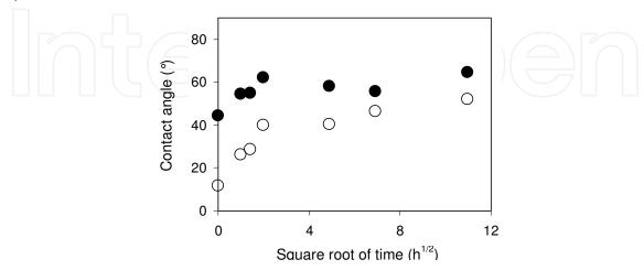
Fig. 10. Contact angle measurements as a function of incubation time in ambient atmosphere performed on  $(\bullet)$  native stainless steel and  $(\bigcirc)$  after UV-ozone treatment.
