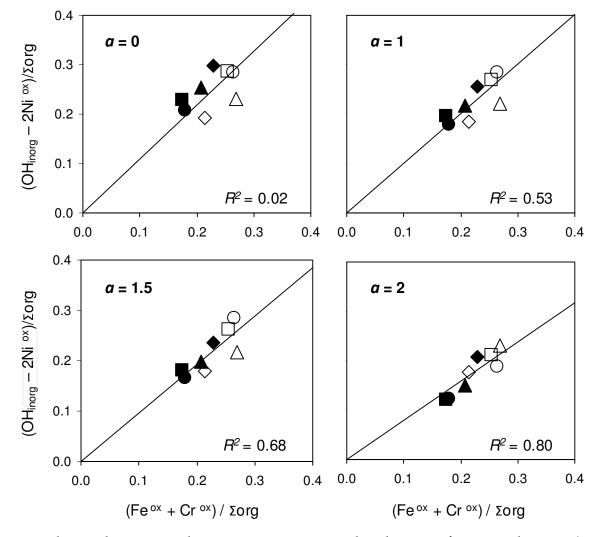
Fig. 7. Relations between molar concentrations ratioed to the sum of organic elements ( $\Sigma$ org) measured by XPS at  $\theta = 0^{\circ}$  (data from Table 2) on native (open symbols) or silanized stainless steel (closed symbols), as such ( $\blacklozenge$ , $\diamondsuit$ ) or further treated with coupling agent BS ( $\blacktriangle$ , $\triangle$ ), glucose oxidase ( $\blacksquare$ , $\bigcirc$ ) or coupling agent followed by glucose oxidase ( $\blacksquare$ , $\square$ ).
