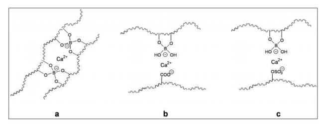
Fig. 4. Proposed mechanisms for the formation of Ulvan-based ionotropic hydrogels through a) Ca<sup>2+</sup> stabilization of borate esters (Haug, 1976) or the participation of b) carboxylate and c) sulphate groups (Lahaye & Axelos, 1993).
