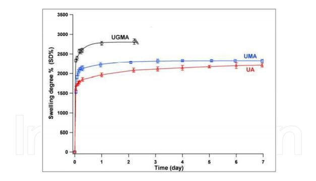
Fig. 10. SD% in PBS buffer solution (0.1 M, pH 7.4) of UV crosslinked (365 nm, approximately  $8 \text{ mW} \cdot \text{cm}^{-2}$ ) UMA and UGMA hydrogels as a function of time.
