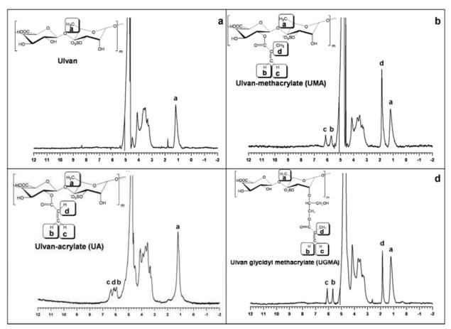
Fig. 6.  $^1$ HNMR spectra in  $D_2O$  of : a) Ulvan, b) Ulvan-methacrylate (UMA), c) Ulvan-acrylate (UA). d) Ulvan-glycidyl methacrylate (UGMA). Chemical structures of the main disaccharide repeating units of the polysaccharides are reported together with the relative peak assignment as highlighted in the small boxes.
