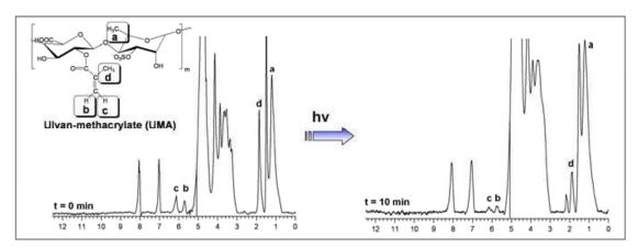
Fig. 9. ¹HNMR spectra of Ulvan-methacrylate (UMA) before and after 10 min of UV irradiation in the presence of IRGACURE® 2959 as photoinitiator. Chemical structures of the main disaccharide repeating units of the macromer is reported together with the relative peak assignment as highlighted in the small boxe.
