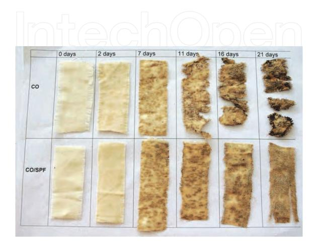
Fig. 11. Fabric samples after having been buried in the soil for 0 to 21 days. (Photo: Marica Starešinič)
