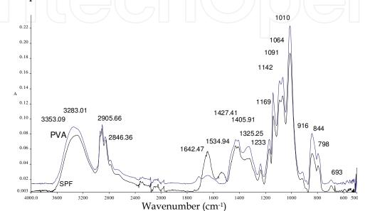
Fig. 6. FT-IR/ATR absorption spectra of soybean protein fibres (SPF) and PVA Kuralon<sup>®</sup>.
