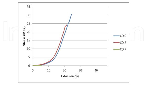
Fig. 13. Stress-elongation curves for cotton woven fabrics.
