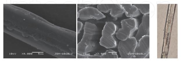
Fig. 5. Scanning electron microscope view of soybean protein fibre: top: longitudinal view at magnification of 4.000 and bottom: cross-section at magnification of 3.000. Right: optical microscope longitudinal view of soybean protein fibre.
