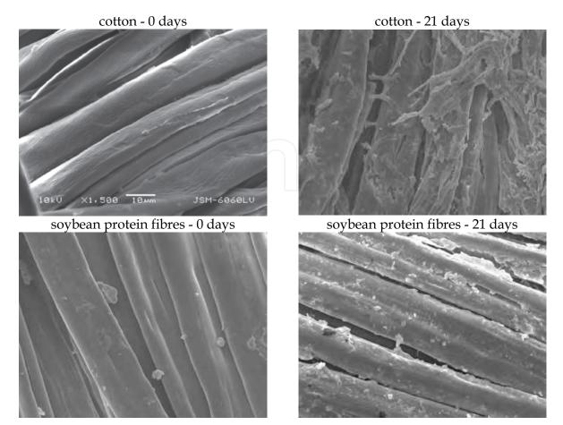
Fig. 12. SEM microphotographs of CO fabrics and SPF/CO woven fabrics (magnification 1500-x).
