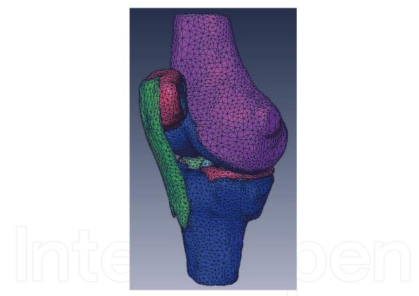
Fig. 10. Mesh of the human knee joint consisting of tetrahedral elements.
