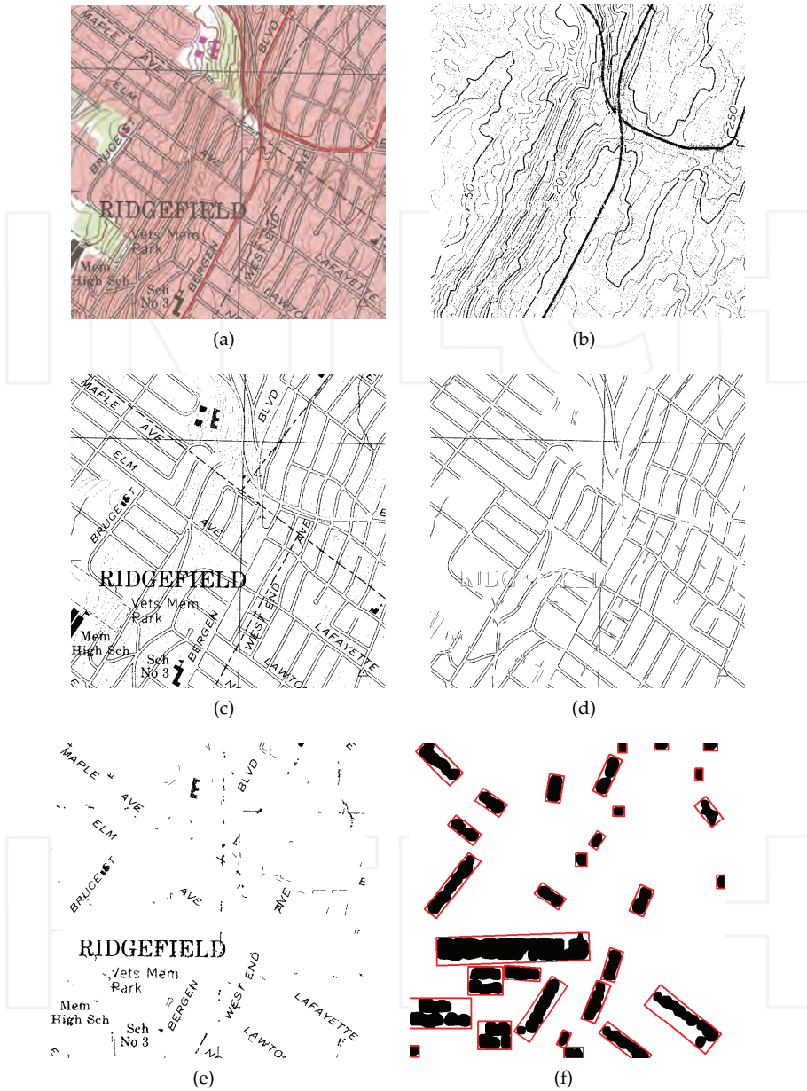
Fig. 1. Performance evaluation of the text and graphics separation modules; (a) Original map image, (b) Extracted Contour Lines, (c) Foreground image, (d) Extracted linear features, (e) Text image, (f) Grouped characters and their respective minimum area enclosing rectangles
