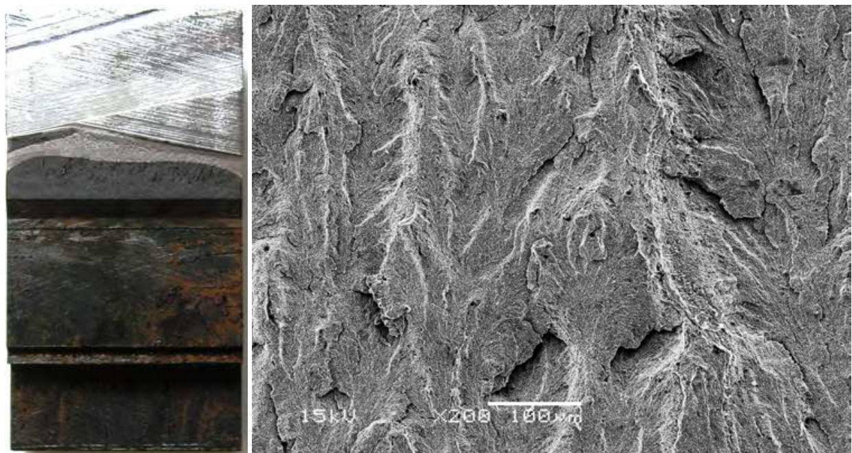
Fig. 11. Morphology of the fracture surface created by SCC, t = 260^{\circ}\text{C} , \text{O}_2 = 4,5 ppm, v_{\text{cor}} = 3,7 \cdot 10^{-5} mm/s
