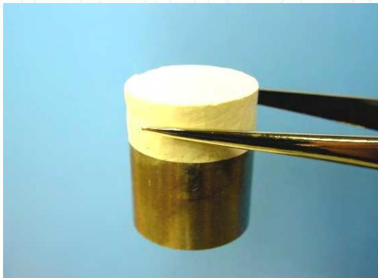
Fig. 4. Photograph of the bonded body of HA ceramics and Ti metal (20mm in diameter).
