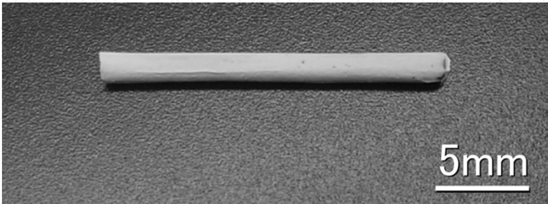
Fig. 15. Photograph of the sample of HA ceramic coating on Ti rod.
