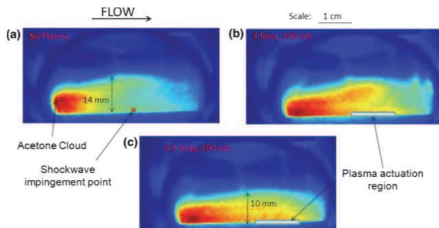
Fig. 17. Time averaged side view of the separation as visualized by acetone PLS with the shock impingement location moved downstream by  $2d$ , (a) base line case with no plasma actuation, (b) plasma actuation at 3 Tesla and (c) plasma actuation at 4.5 Tesla [Karla et al, 2010].
