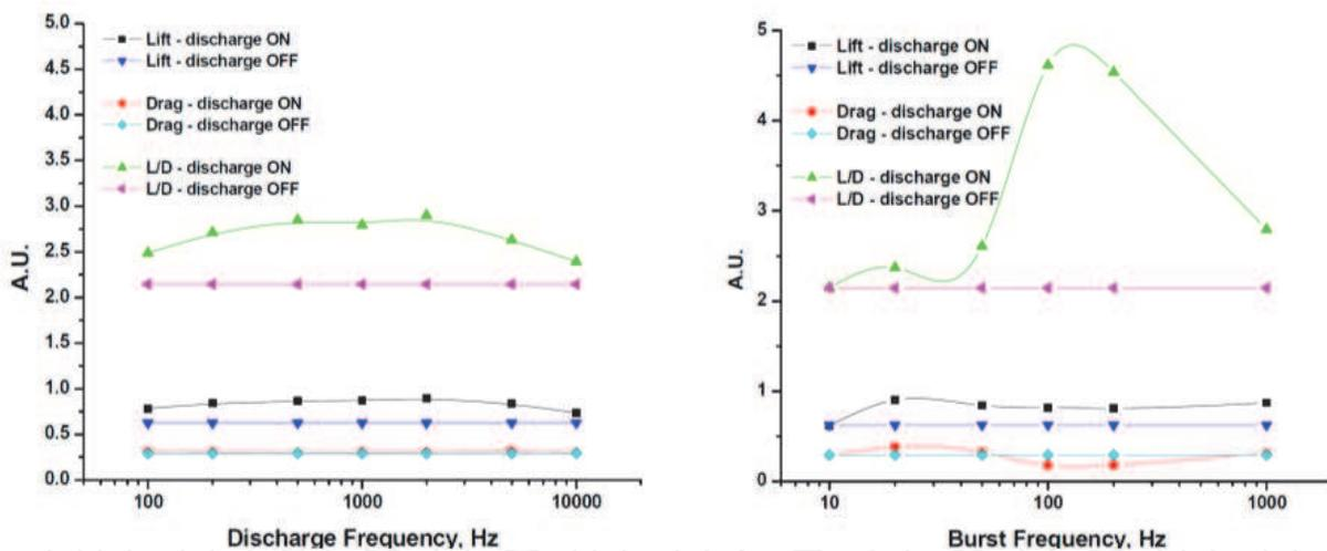
Fig. 36. Lift, Drag force and Lift-to-Drag ratio in dependence on the frequency.  $\alpha = 22^\circ$ ;  $U^\infty = 17.4$  m/s; a) - Periodic Mode,  $P = 2.5$ -250 W for  $f = 100 - 10000$  Hz, respectively; b) - Burst Mode,  $P = 25$  W for all regimes [Sidorenko et al, 2007].
