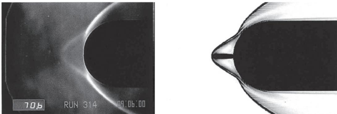
Fig. 14. a) Schlieren picture of counter-flow experiment. b) Calculated flow patterns of counter-flow configuration [Shang, 2002].
