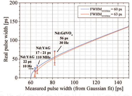
Fig. 4. Calibration curves for our measuring photodiode-oscilloscope system (for FWHM<sub>SYSTEM</sub> of 60 and 63 ps) and calculated real pulse durations of three measured laser sources
