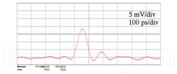
Fig. 1. Oscilloscope trace of the measured 2 ps long pulse using sin(x)/x approximation.
