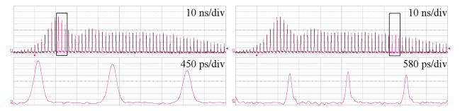
Fig. 8. Nd:YAG laser system output pulse train oscillogram (upper traces) and details of the pulse shapes from the beginning and end of the train (lower traces).
