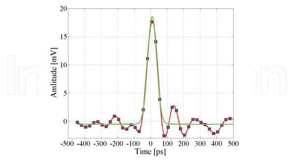
Fig. 2. Measured 2 ps long pulse (dots) and its Gaussian fit (green line) and Spline fit (red curve).
