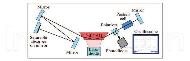
Fig. 3. Schematic of the Nd:YAG laser system generating  $22 \pm 2$  ps pulses.
