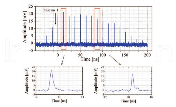
Fig. 6. Nd:GdVO<sub>4</sub> laser system output pulse train oscillogram (upper trace) and zoomed pulses no. 3 and 9 (lower traces).
