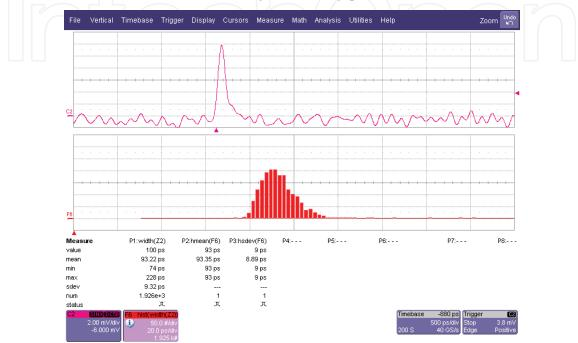
Fig. 5. Single pulse stability investigation using the oscilloscope statistical functions. Upper trace: measured pulse, lower trace: pulse width histogram from  $\sim$  2000 successive pulses.
