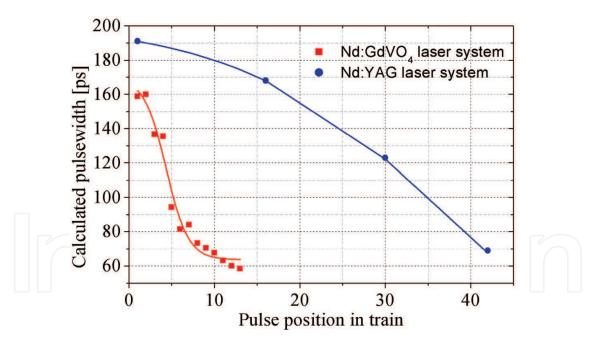
Fig. 7. Calculated pulse duration evolution along the trains generated by the Nd:GdVO<sub>4</sub> and Nd:YAG laser systems.
