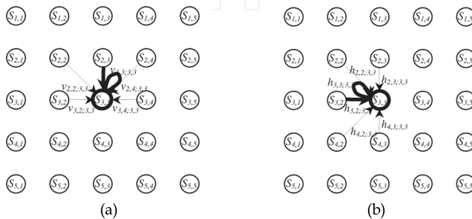
Fig. 14. Modified LC2D HMM [Othman & Aboulnasr, 2003]. (a) Vertical transitions to state S_{3,3} for 5x5 state model (b) Horizontal transitions to state S_{3,3} also for 5x5 state model.
