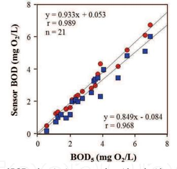
Fig. 13. Comparison of BOD values in river waters by with and without ozonation in the stopped-flow system. ■: without ozonation, ●: with ozonation.
