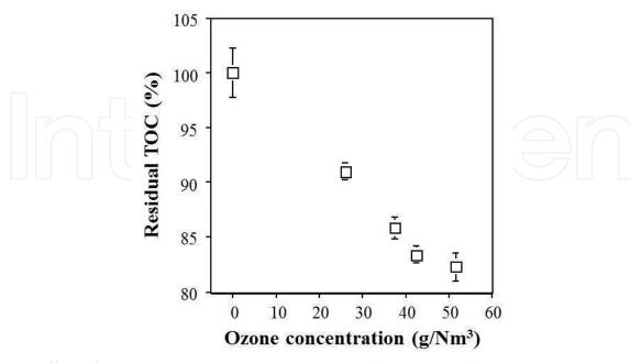
Fig. 12. Effect of ozone concentration on TOC removal in AWW solutions. Pretreatment time: 3 min, pH: 7.0, temperature: room temperature.
