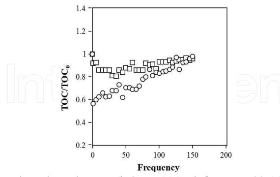
Fig. 8. Photocatalytic oxidation rates of TiO<sub>2</sub> using AWW in the flow system. TOC<sub>0</sub>: AWW non-through a photoreactor, TOC: AWW through a photoreactor,  $\Box$ : without irradiation,  $\circ$ : with irradiation (*i. e.* pretreatment by potocatalysis.).
