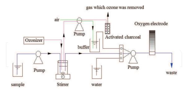
Fig. 9. Schematic diagram of the stopped-flow system of the BOD sensor using pretreatment with ozone.
