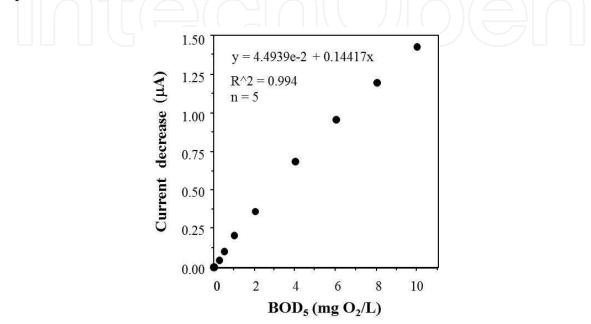
Fig. 1. Correlation between BOD concentration and current decrease using the AWW solution under the optimal conditions.
