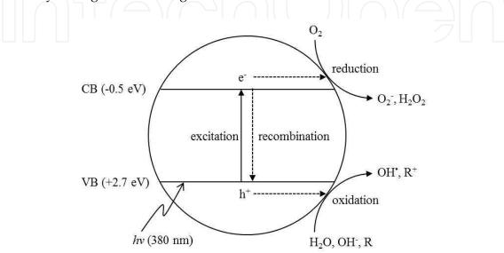
Fig. 5. Schematic diagram of simplified mechanism for the photoactivation of a titanium dioxide particle.
