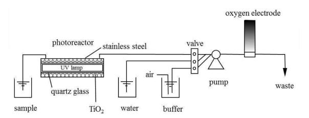
Fig. 6. The photocatalytic BOD sensor of the flow system using pretreatment by photocatalysis. A column size: ID 22 x OD 34 x L 205 mm, total volume: 63 mL, amount of TiO<sub>2</sub>: 47 g, a UV lamp: a 6W black, flow rate: 3 mL/min.
