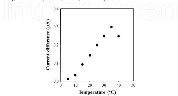
Fig. 3. Influence of temperature on the sensor response at pH 7.0 and AWW (1 mg/L BOD).
