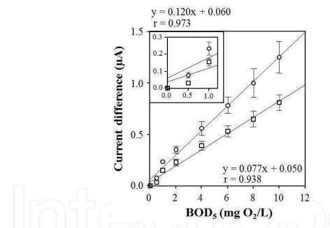
Fig. 10. The sensor responses before and after ozonation in the stopped-flow system under the optimal conditions.  $\Box$ : before ozonation,  $\circ$ : after ozonation.
