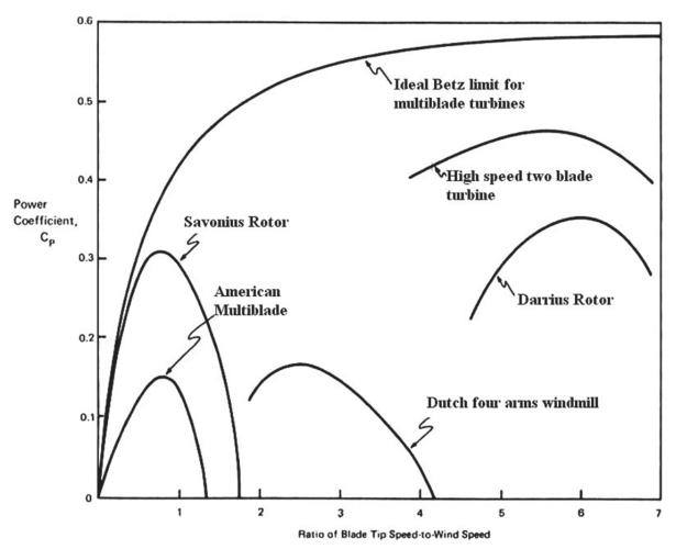
Fig. 6. The power coefficient C<sub>p</sub> as a function of the tip speed ratio for different wind machines designs. Note that the efficiency curves of the Savonius and the American multiblade designs were inadvertently switched (Eldridge, F. R., 1980) in some previous publications, discouraging the study of the Savonius design.
