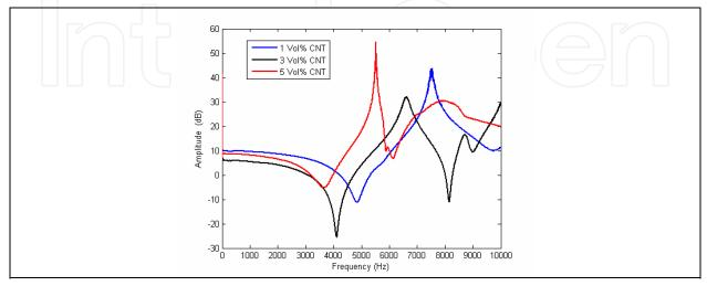
Fig. 6. Measured frequency response function from excitation of the specimens
