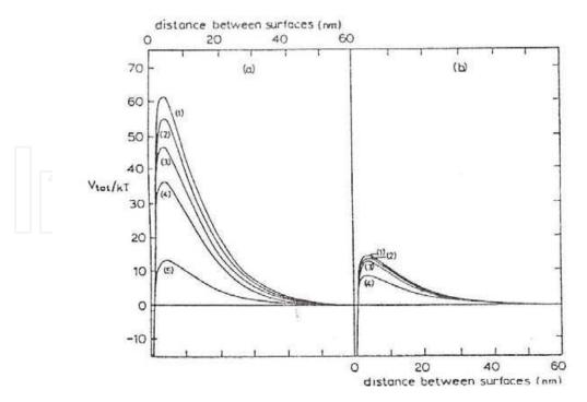
Fig. 4. Theoretical curves of total potential energy against distance of separation of two spherical particles of radii  $a_1$  and  $a_2$  and equal surface potential (35.86 mV);  $1/k = 10^{-6}$  cm (from Parfitt 1981)
