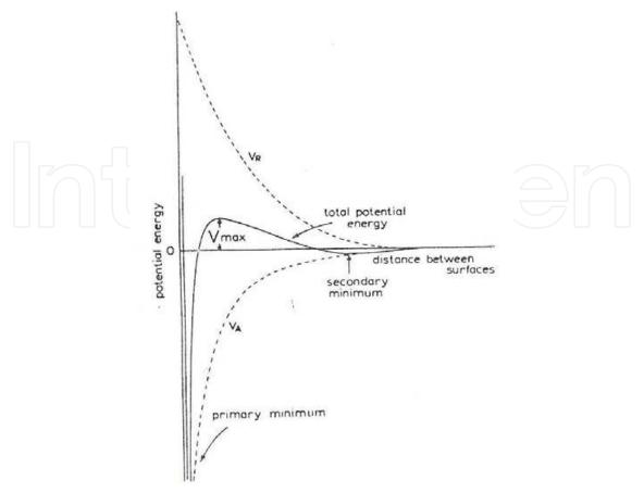
Fig. 2. DLVO potential representation:  $V_A$ : attractive Van der Waals potential;  $V_R$  repulsive electrostatic potential (from Parfitt 1981)
