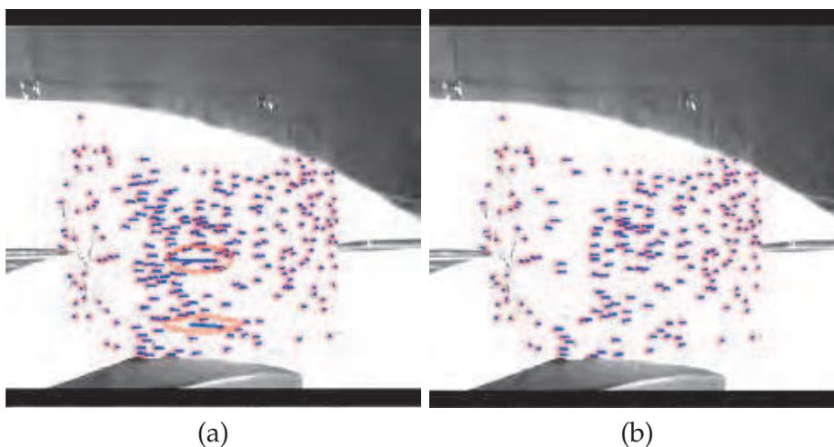
Fig. 12. Optical flow extraction before (a) and after (b) eliminating undesired paired points.
