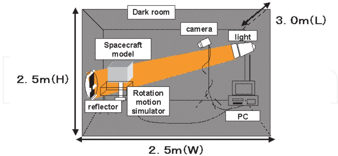
Fig. 1. Schematic representation of the in-space lighting simulator.
