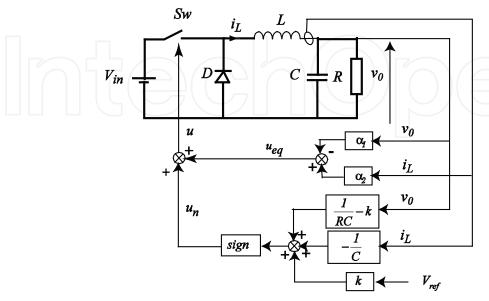
Fig. 4. SMC for Buck converter
