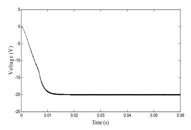
Fig. 12. Output vvoltage evolution obtained by application of the SMC
