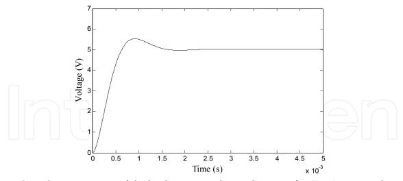
Fig. 7. Open loop responses of the buck converter by application of 16% PWM control signal
