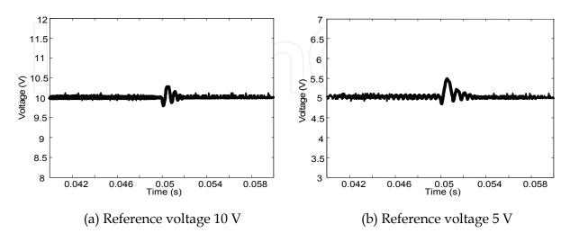
Fig. 26. Experimental test robustness of the FSMC for the variation of the load from 10  $\Omega$  to 15  $\Omega$
