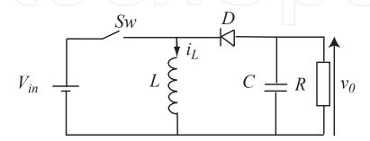
Fig. 3. Buck-Boost converter structure
