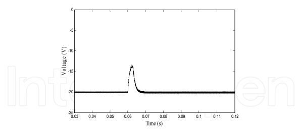
Fig. 14. Output voltage evolution by application of the SMC for the case of load variation from  $30\Omega$  to  $20\Omega$
