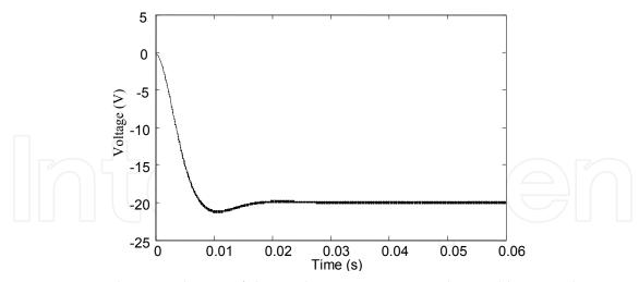
Fig. 11. Output voltage evolution of the Buck-Boost converter obtained by open-loop control.
