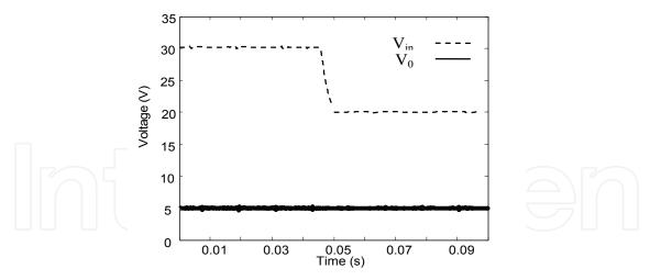
Fig. 27. Experimental output voltage evolution by application of the FSMC for the variation of the input voltage from 30V to 20V
