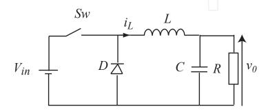
Fig. 1. Buck converter structure
