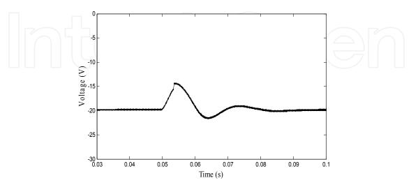
Fig. 31. Output voltage evolution by application of the SMC for the case of input voltage variation from 15 V to  $10\mathrm{V}$
