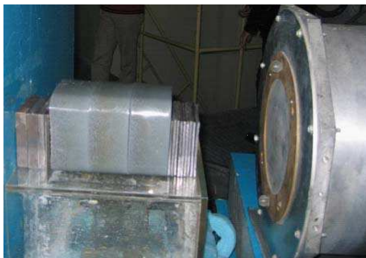
Fig. 22. The measurement of Sample neutrons shielding materials absorption
