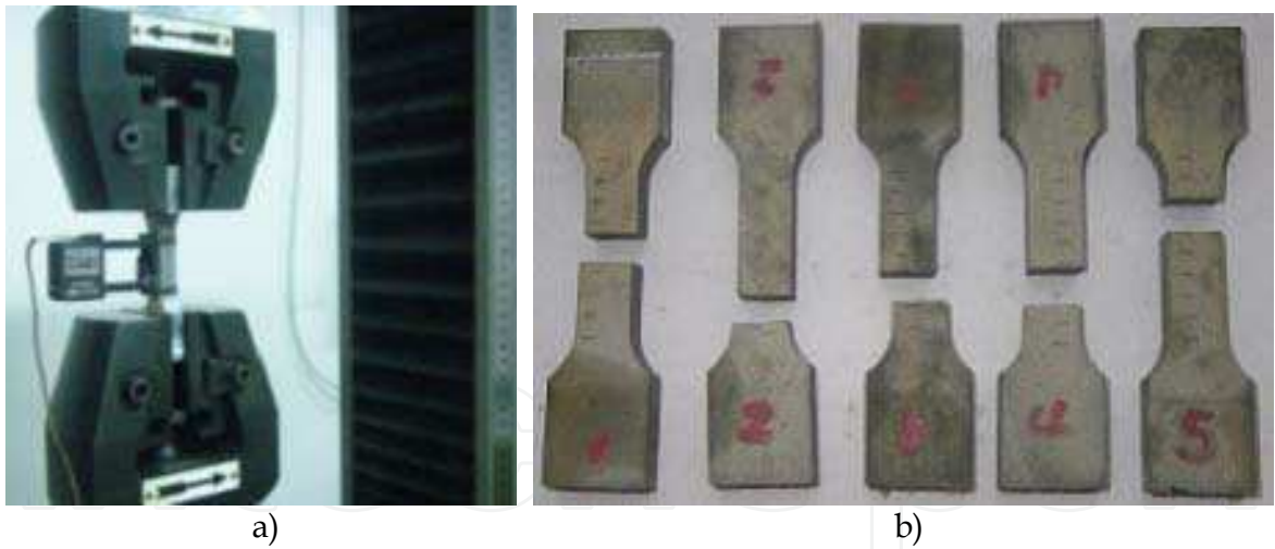
Fig. 28. The determine experiment of the samples Jxa1(including tensile rate) a) The draw experiment of Jxa1 b) the broken experiment sample of Jxa1
