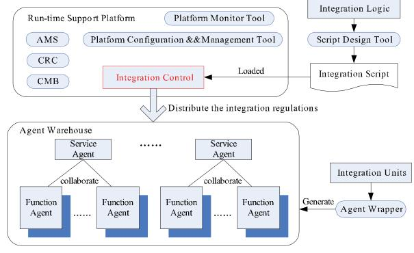
Fig. 6. Architecture of ASIDE
