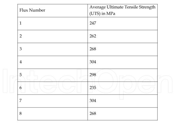
Table 12. Experimental Results for the Ultimate Tensile Strength (UTS) Test
