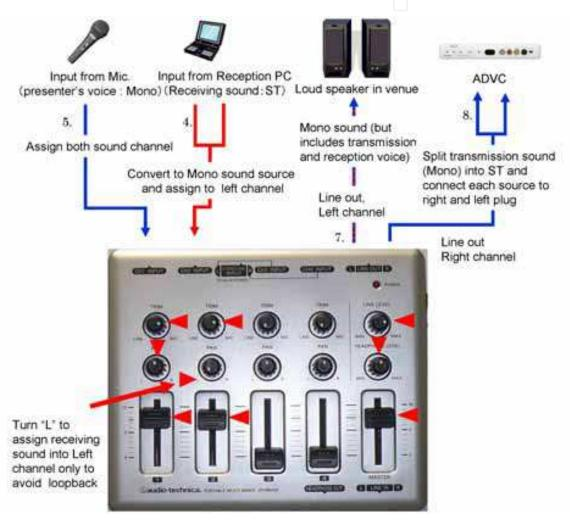
Fig. 4. Configuration diagram for setting audio
