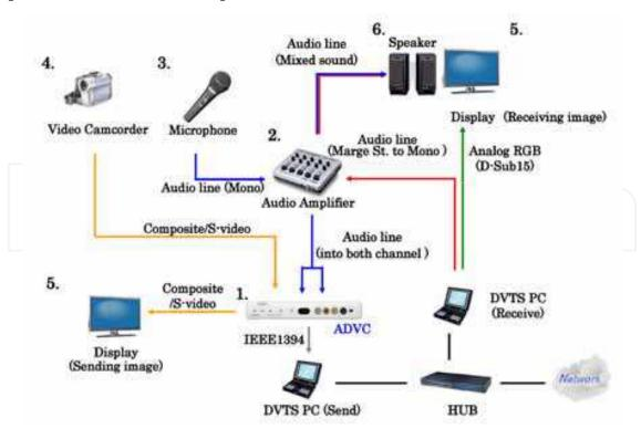
Fig. 3. Standard configuration: 1. Analog-Digital Video Converter (ADVC), 2. Audio amplifier, 3. Microphone, 4. Video camera, 5. Display, 6. Loud speaker
