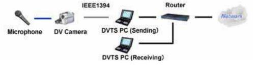
Fig. 2. Minimal configuration for DVTS setup
