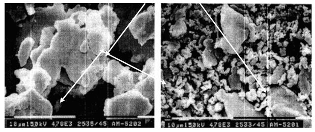
Fig. 6. SEM Micrographs illustrating contact between silver flakes
