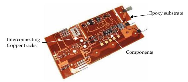
Fig. 1. Populated Printed Circuit Board
