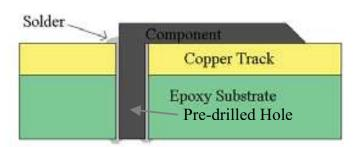
Fig. 4. Through Hole Component
