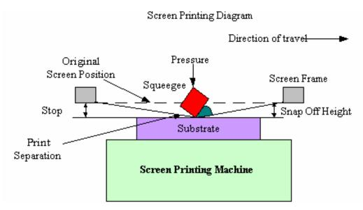
Fig. 11. Screen Printing Process
