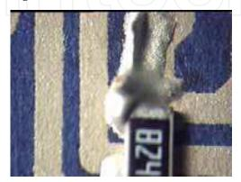
Fig. 22. ECA Spreadage after Printing
