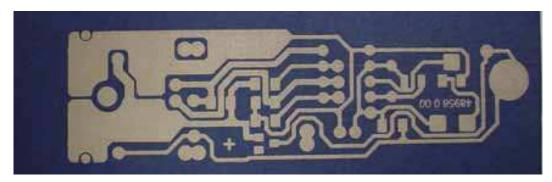
Fig. 15. Successful printing of Conductive ink
