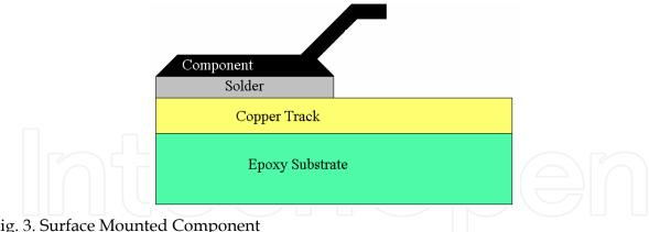
Fig. 3. Surface Mounted Component
