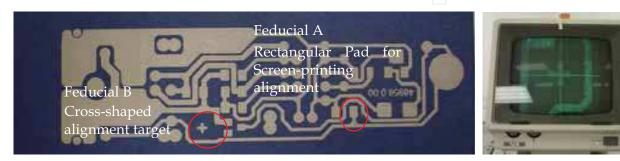
Fig. 18. Feducial used for Vision Alignment
