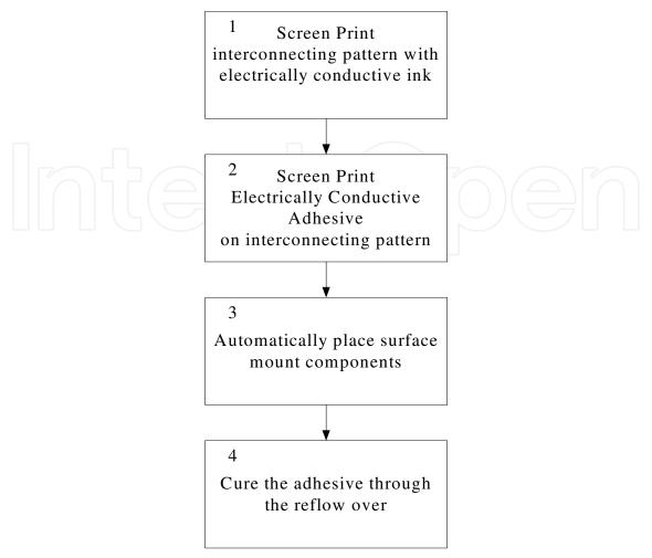
Fig. 12. The Manufacturing Process
