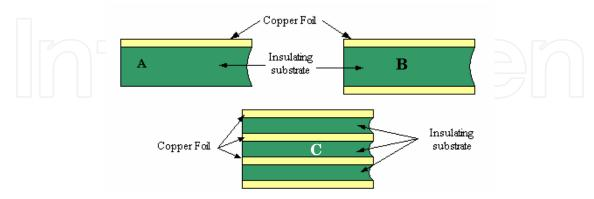
Fig. 2. Three types of PCB structure, (a) Single-sided, (b) Double sided and (c) Multilayer
