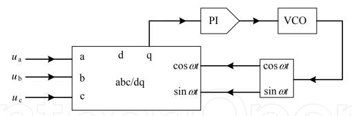
Fig. 16. Block diagram of the synchronization circuit
