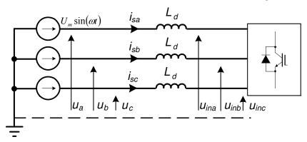
Fig. 14. Diagram of the rectifier connection to a supply network
