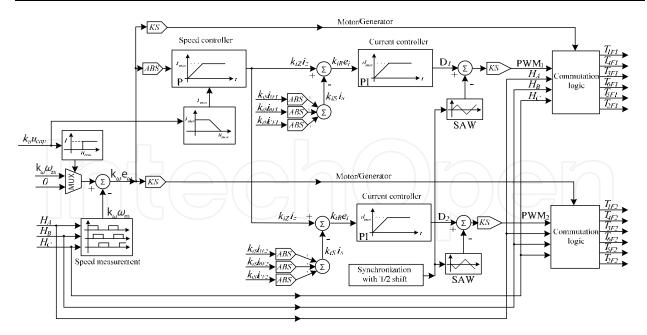
Fig. 28. The inverters' control system
