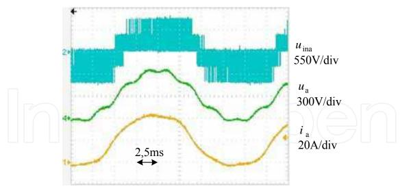
Fig. 21. The waveforms of the phase voltage and current  $u_a$ ,  $i_a$  and the input voltage  $u_{ina}$  in phase A
