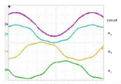
Fig. 17. The synchronizing voltage waveforms and the generated function cos ωt
