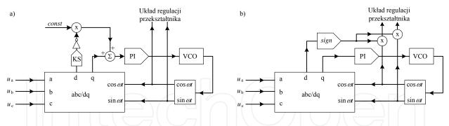
Fig. 19. Two versions of the synchronizing circuit enforcing the correct generation of  $\cos \omega t$  function
