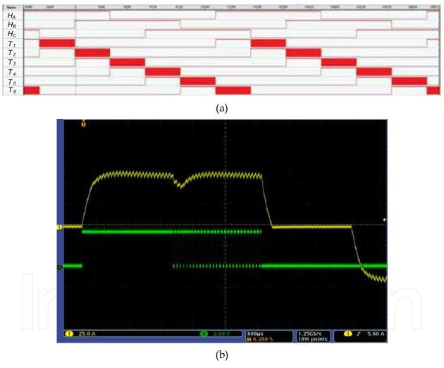
Fig. 31. a) Hall sensors signals and transistors gate control pulses; b) The motor phase current and transistor gate control pulses limiting switching losses
