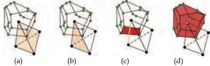
Fig. 5. Duality between VD and DT in 3D
