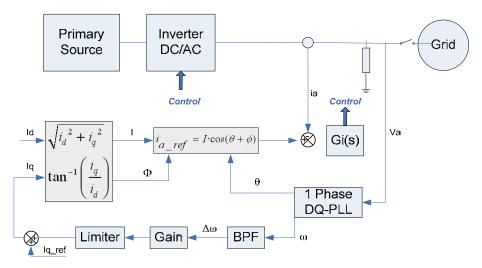
Fig. 13. Block diagram of the GEFS method
