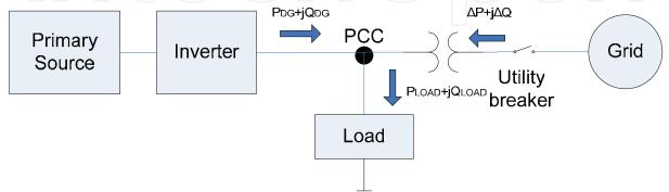
Fig. 3. Power balance in a local load supplied both by the grid and a distributed generator
