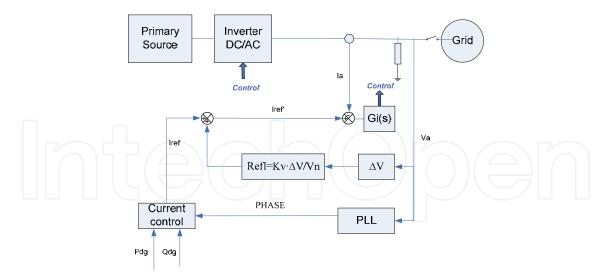
Fig. 12. Block diagram of the SVS method
