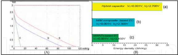
Fig. 10. Galvanostatic discharge curves (A) and energy density at 10 mA/cm<sup>2</sup> current density (B) of (a):  $MnO_2$  / MWNT – MWNT asymmetric capacitor, (b):  $MnO_2$  / MWNT –  $MnO_2$  / MWNT symmetric capacitor, and (c): MWNT – MWNT symmetric capacitor (Wang et al., 2005).
