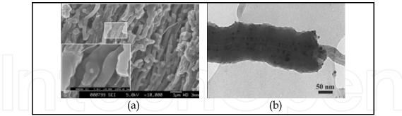
Fig. 6. Polypyrrole coated aligned MWNTs (polymerization charge ~ 40 C/cm<sup>2</sup>, nanotube length ~ 100  $\mu$ m). (a): SEM image of the fractured film cross section illustrating the thickness of the polypyrrole coating relative to the uncoated MWNTs, exposed by fiber-pullout, as well as the channels available to the electrolyte between the coated nanotubes. (b): TEM image showing good interaction between the polypyrrole and MWNT (Hughes, et al., 2002 (*Adv. Mater.*)).
