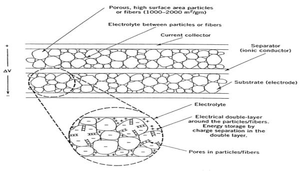
Fig. 1. Schematic of an electrical double-layer supercapacitor (Burke, 2000).
