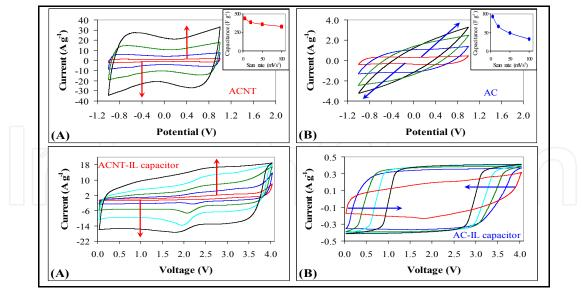
Fig. 13. TOP: CVs obtained in  $[EMIM][Tf_2N]$  for an aligned CNT electrode (A) and an activated carbon electrode (B) at 5, 20, 50, 100 mV/s as indicated by arrows. Insets show capacitance change of the electrodes upon the increase of scan rate. BOTTOM: CVs obtained for an aligned CNT capacitor (A) and an activated carbon capacitor (B), both fabricated from ionic liquid (IL)  $[EMIM][Tf_2N]$ , at the scan rate increasing from 5, 20, 50, 100 mV/s as indicated by arrows (Lu et al., 2009).
